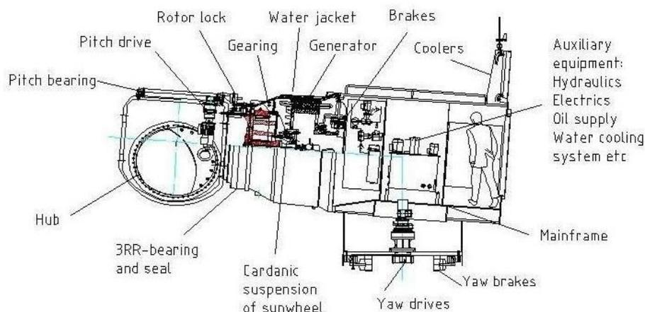
Fig. 1 Cross section of the WWD1
